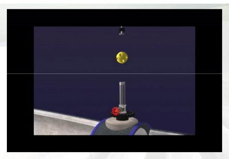
The rolling ball listens for leaks from *inside* the pipe...
